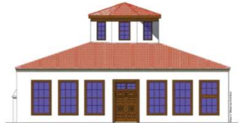
Reconstruction elevation drawing of Beth El synagogue in Komotini, Northern Greece. The synagogue was surveyed in 1993 prior to its demolition in April 1995. © Elias Messinas
